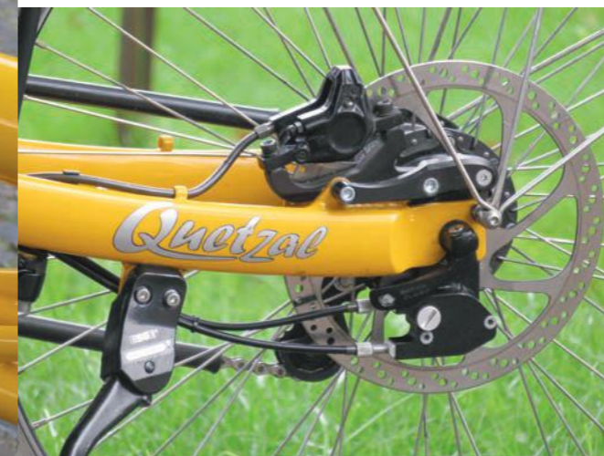
Large disc on rear swing-arm too, solid plate for kickstand fixation, external Rohloff gear-box.
